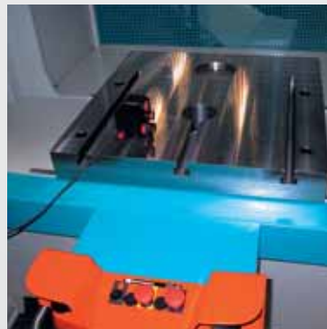
Special bed plate with die cushion
