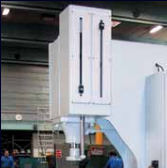
Cam control – top- and bottom stop
